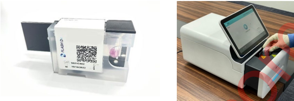
Figure 3. Left: Fully closed sample port lid is flush with the rest of the cartridge top. Right: Load the cartridge into the instrument's loading bay.
